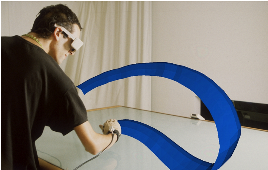
Figure A.20: “Surface drawing” by Schkolne et al: hand motions create 3D shapes which “float” over the Responsive Workbench
