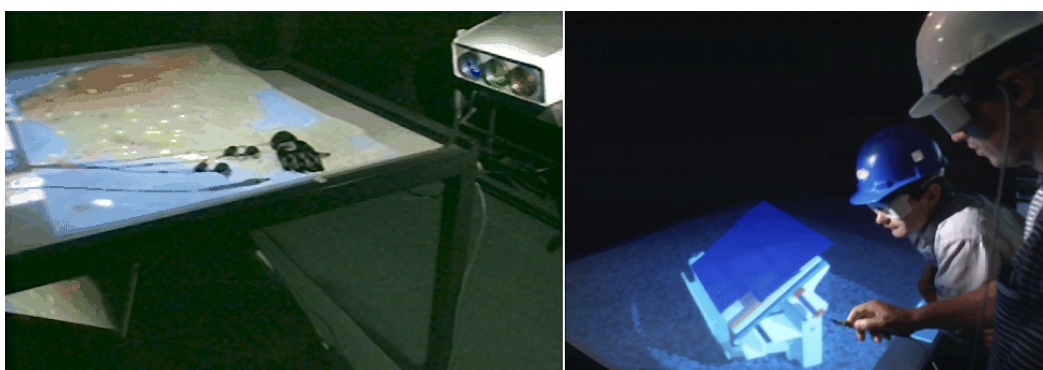
Figure A.15: Responsive Workbench: stereo video projected on mirrors below the desk (left), and persons observing a 3D house model displayed in stereo (right)
