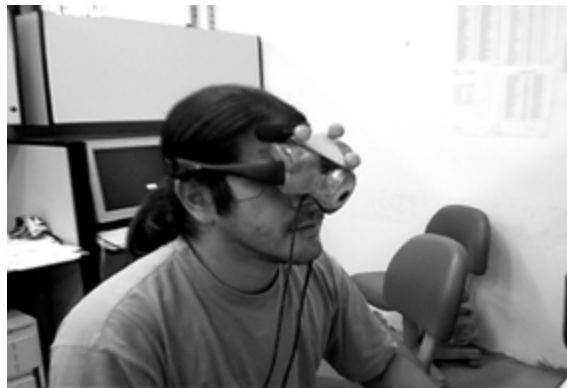
Figure 4. A user wearing an HMD with a webcam attached.
